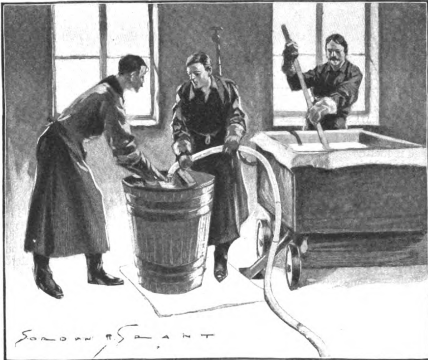
WASHING THE GOLD, AFTER THE SILVER AND THE COPPER HAVE BEEN DISSOLVED WITH SULPHURIC ACID—THE SQUARE BOX ON THE RIGHT CONTAINS ABOUT FIVE HUNDRED THOUSAND DOLLARS' WORTH OF GOLD DUST.
